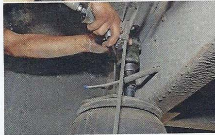
2, 3. The lower air bag mounting nuts are removed first, followed by the upper mounting nuts. Then the bag is removed.
