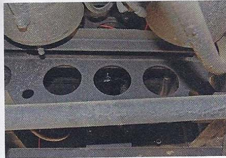
6. A front cross member on the R4R and R4RR chassis is an ideal spot for the Source Engineering ping tank.
