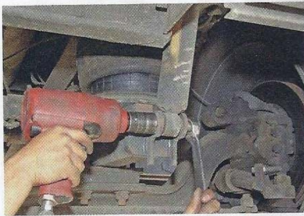
1. The stock front shock absorbers are removed and discarded, as they will be replaced with new Bilstein shock absorbers designed specifically for the REK-202 Ride Enhancement Kit.
