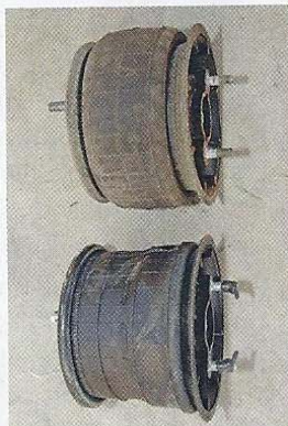
2, 3. The lower air bag mounting nuts are removed first, followed by the upper mounting nuts. Then the bag is removed.
