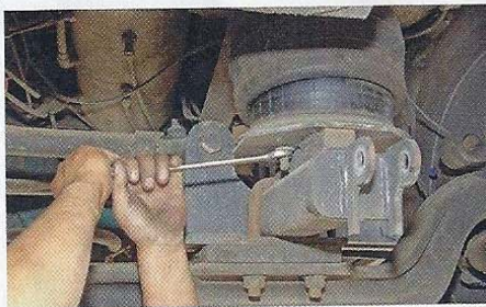
1. The stock front shock absorbers are removed and discarded, as they will be replaced with new Bilstein shock absorbers designed specifically for the REK-202 Ride Enhancement Kit.
