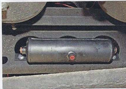
7. To mount the ping tank, a bracket is placed behind the cross member, and the fastener placed through mounting tabs on the ping tank. No drilling is required.
